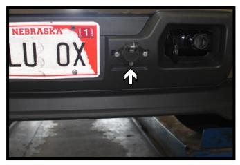
13. **Optional:** Prior to fully reinstalling the fascia. Drill a hole thru the bumper at the deisired location to accomodate the plug and bolts. Using 1/4" x 1-1/2" bolts with 1/4" washers, install the plug thru the bumper. On the backside of the bumper, install the electrical bracket and 1/4" locknuts to secure the plug to the bumper.
