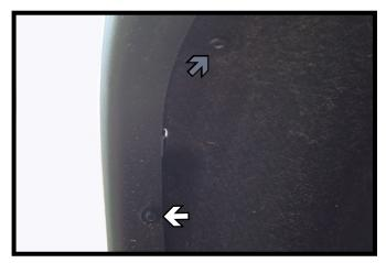
4. Using a 7MM socket, remove the screw from the wheel well (white). Using a T15 Torx, remove the upper screw (gray). Do this on both sides of the vehicle. Unsnap the fascia from the body and set aside.
