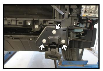
Using a 15MM socket, remove the three
