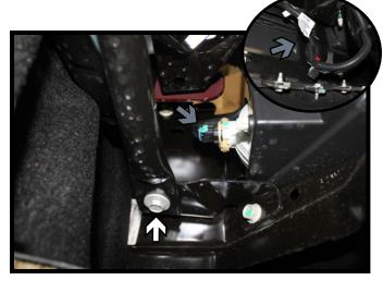
Using a 15MM socket, remove the bolt from the bumper reinforcement bar.
