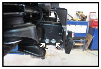
Using a 18MM socket/wrench, remove the two (2) bolts from the tow hook. Do this on both sides of the vehicle.
